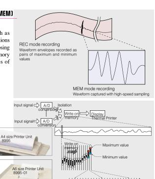
Because of this, the volume of recorded data is compressed while following steep fluctuations of the measured input voltage. Note: When data recorded with the Recorder function is viewed on a PC, both minimum and maximum values appear as a time series of data points.
